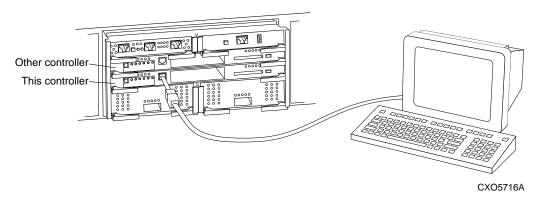
Figure 2–6. "This Controller" and "Other Controller"
